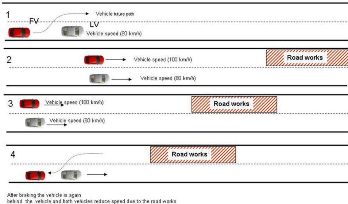
Fig. 5. Illustration of Scenario 2: overtaking on roads with unknown road works
