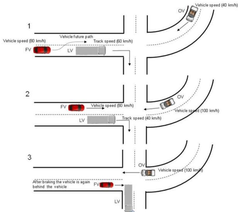
Fig. 4. Illustration of Scenario 1: overtaking on roads with unknown curves and oncoming and turning traffic
