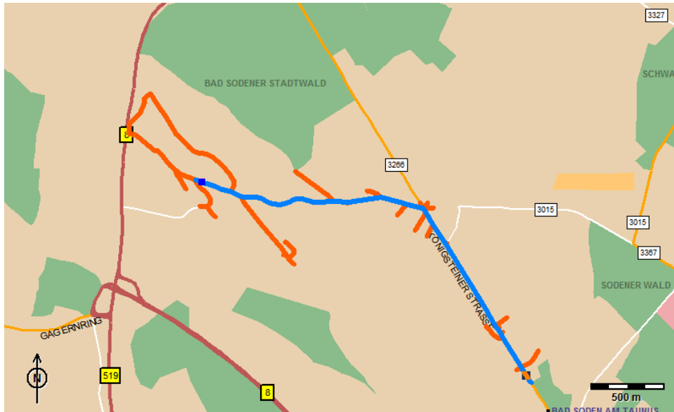
Figure 4. Electronic Horizon (orange) & Most Probable Path (blue)
