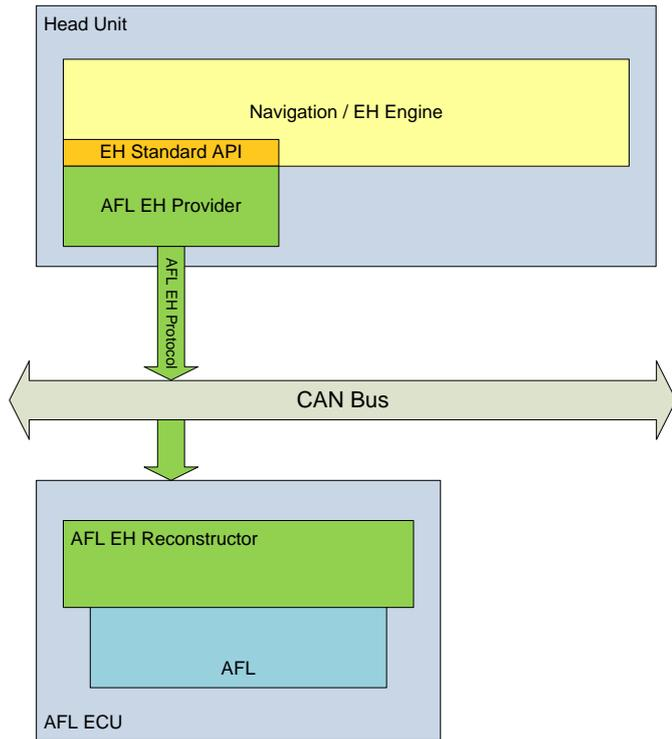
Figure 9 AFL on ECU, AFL-specific protocol
