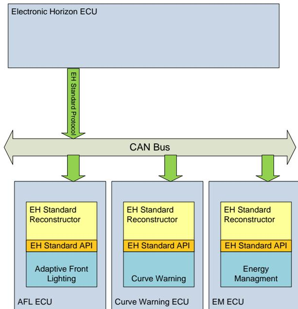
Figure 12 Multiple ADAS with EH ECU
