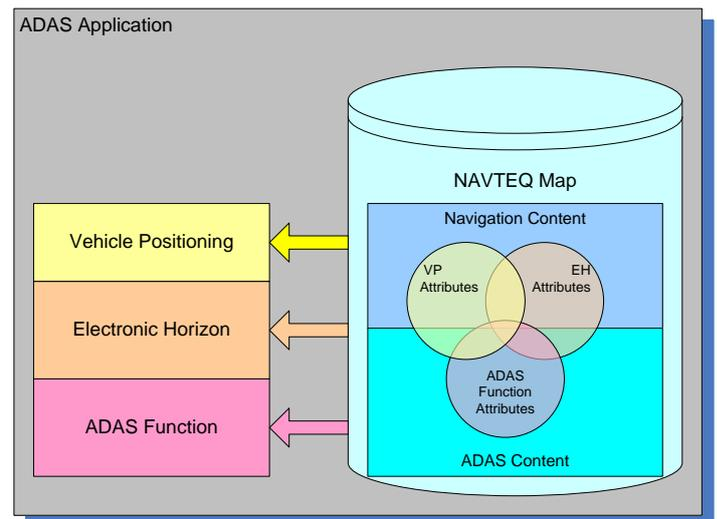
Figure 1 Main Components of the Map-Supported ADAS
