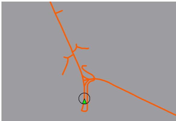
Figure 3 Electronic Horizon (red) in the Digital Map
