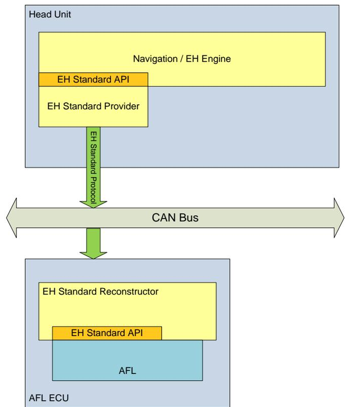
Figure 10 AFL on ECU, standard EH protocol and API
